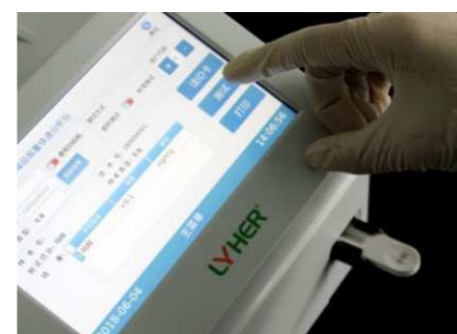
7.Insert test kit immediately into the analyzer after 3-minute reaction. Click "Test" to get drug concentration result
