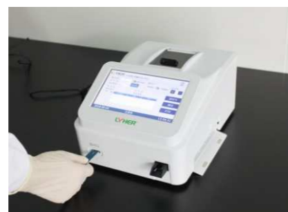
2.Remove the ID card and insert it into analyzer, click "Read ID Card" detect the test kit after finishing the reading
