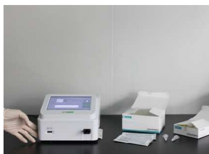
1.Remove and place the analyzer horizontally, connect power adapter, turn on the left switch and right card slot. Remove hair lysate and test cassette, let them return to room temperature
