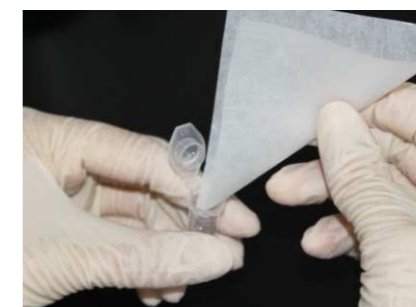
5.Pour shredded hairs into a bottle containing hair lysate, cover the cap, shake for 1 minute
